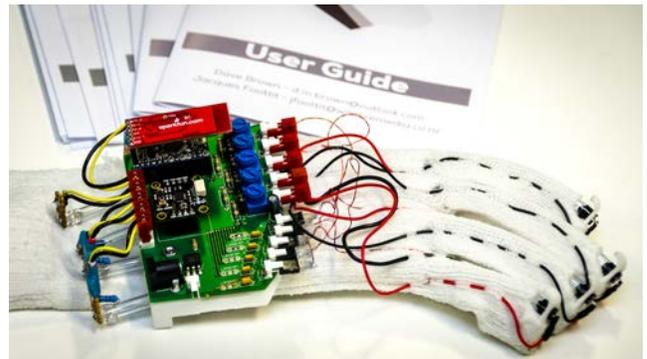
**Figure 1. The final haptic glove.**
