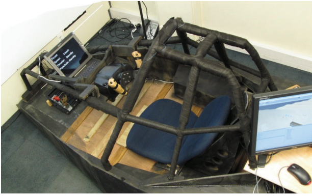
Figure 2: Components of our simulator: Screen (top left), cockpit with yoke (centre) and computer running the vehicle simulation (bottom right).
