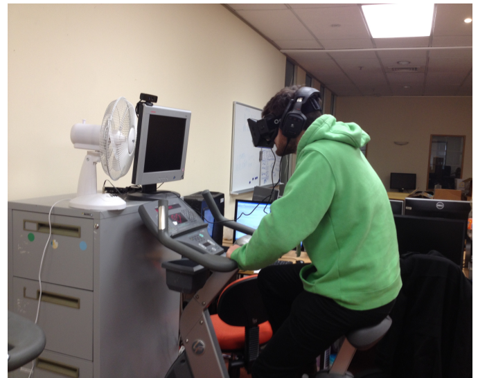
Figure 12: User on the exercise bike, wearing the Oculus Rift and headphones. The depth camera is visible in front of the user.
